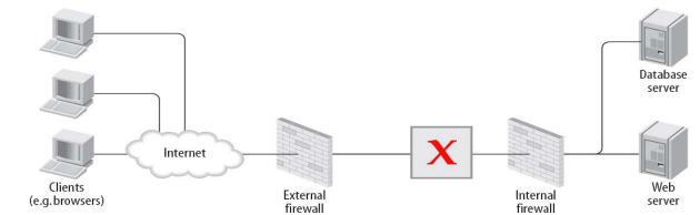
Figure 1. Deployment of the WAF in the web server infrastructure as well as external reverse proxy server
